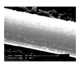
Fig1: TEM micrograph of a glass fiber sized with SIZICYL<sup>TM</sup> XC R2G formulation
