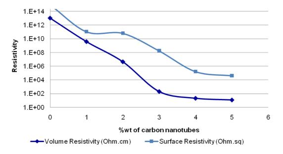
N.B.: Electrical resistivity measurement in accordance to CTM E043 and CTM E402 (Cabot Testing Method), on standard injection molded IZOD specimens.
