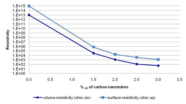
N.B.: Electrical resistivity measurement in accordance to CTM E043 and CTM E402 (Cabot Testing Method), on standard injection molded IZOD specimens, processed according to parameters provided before (General Processing Guide for Injection Molding).
