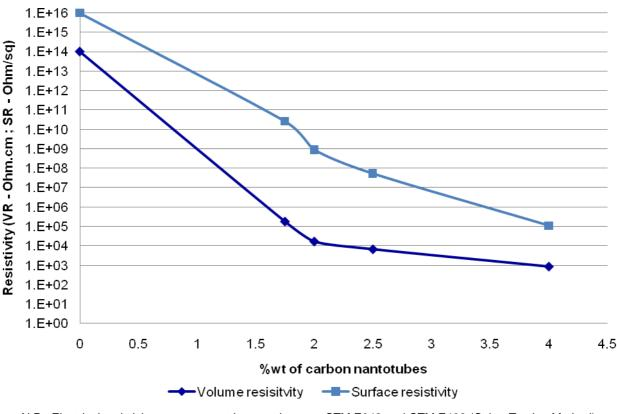
N.B.: Electrical resistivity measurement in accordance to CTM E043 and CTM E402 (Cabot Testing Method), on standard injection molded IZOD specimens.
